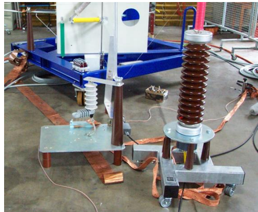
Impulse current testing arrangement for MV arresters
