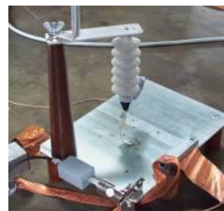
Impulse current testing arrangement with SSG ZUB
