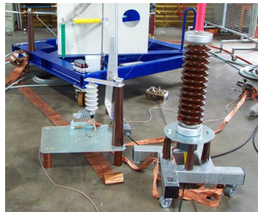
Impulse current testing arrangement for MV arresters
