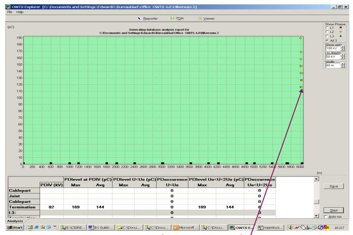
L1, L2 : up to 2xUo PD free (PD < 10 pC)/ L3 : PDIV @ 82kV; PD level ~ 180 pC located in the termination
